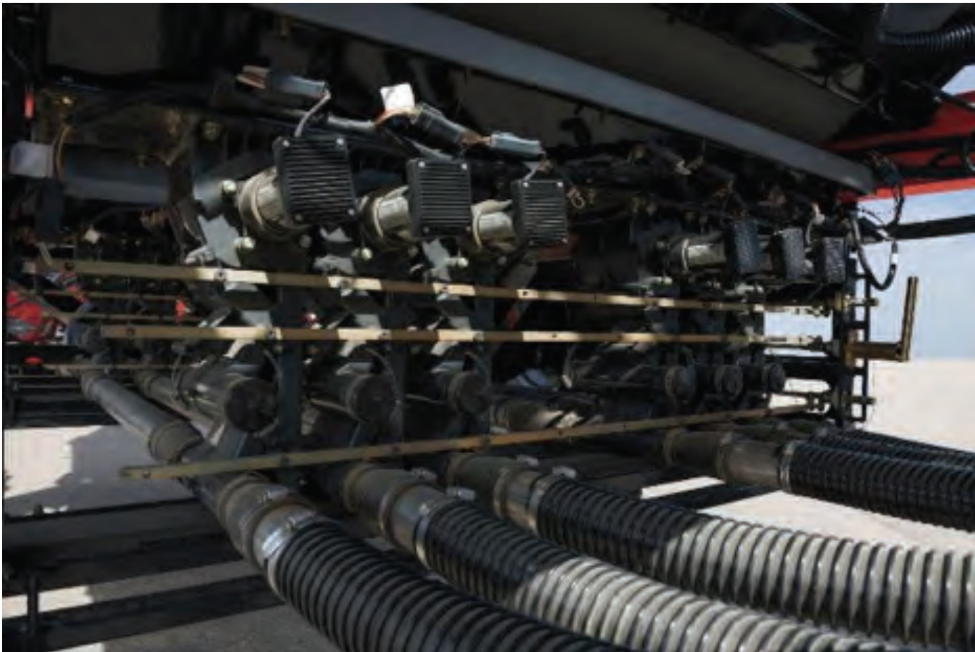
The 5-series air cart feature a modular metering design
