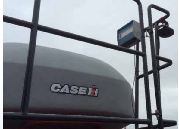
Bulk-Fill Weigh Scale for Monitoring Seed Tank Level
