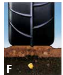
F Verify press wheel (if equipped) function ( F ).
