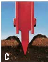
C Check furrow forming point depth ( C ).
