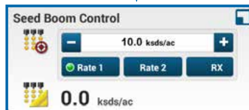
Seed Boom Rate Control – Utilizes the rates or prescription defined in the AFS Pro 1200 Product Setup. UDW is active when Task Controller is selected.
